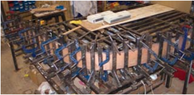
Laminating the inner stem needed all the clamps we could find.
