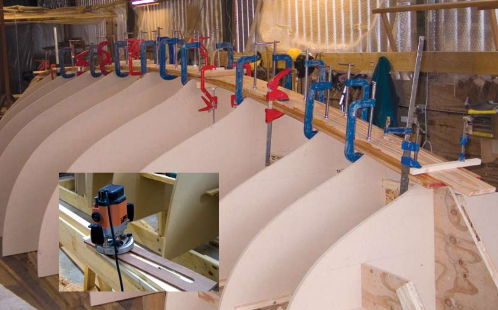
Laminating the inner keel in situ over the building moulds. The inset shows the jig we made for scarphing the strip planks with the router.
