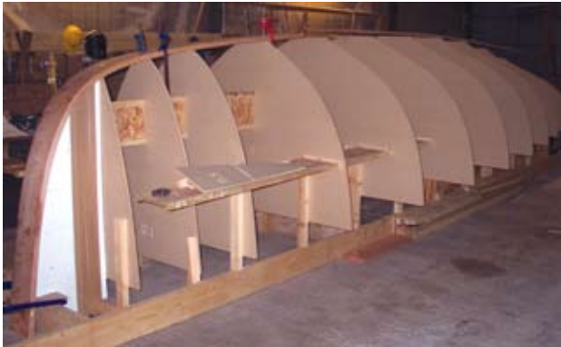
The laminated inner stem – apron – in position on the building jig.
