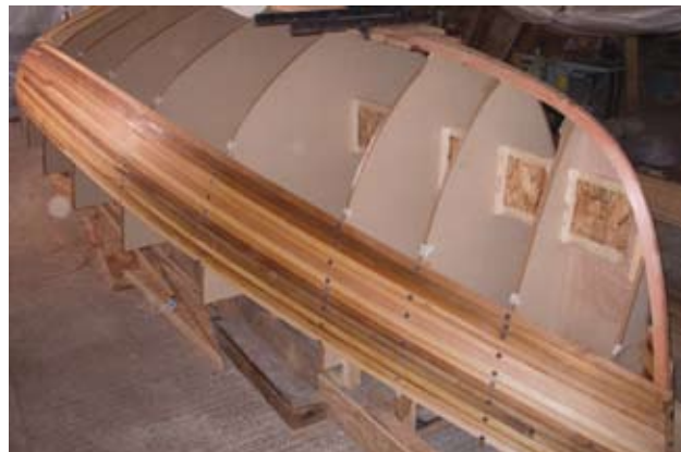
Robbins' Rapid Strip is self-locating which speeds up progress.
