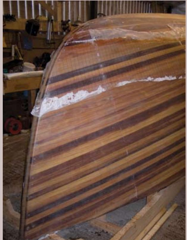
without it running off, before the cloth is applied and the remaining resin is used to wet out any dry areas after pressing the cloth in place with rollers.
