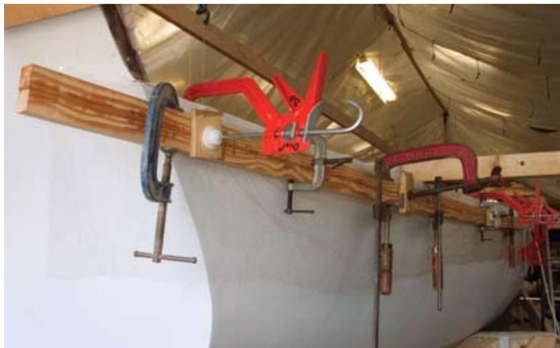
boatbuilding, we turned to the properties of epoxy resin again and made the section out of two pieces of Douglas fir laminated one above the other. The hull itself makes the ideal laminating jig. After we taped some polythene along the sheer we cramped the laminates around the outside following the horizontal curve perfectly.
