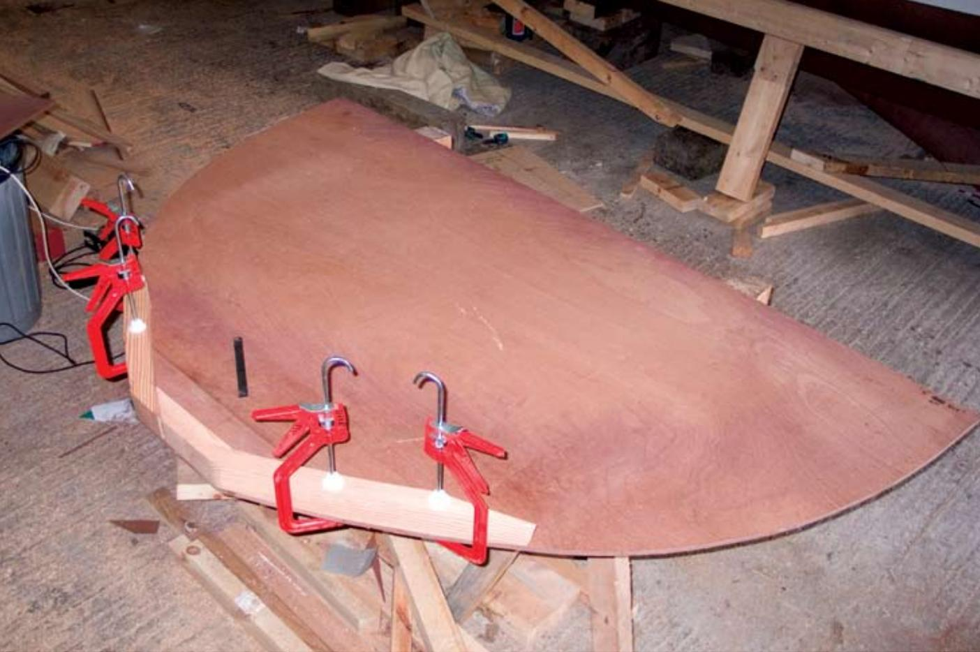
*The keelbolts were positioned to go in pairs through wooden floors like this one, fabricated at the base of each of the plywood bulkheads.*
