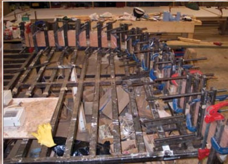
**Background picture:** First frame in place. **Above:** Removing the moulds, glueing the laminates, laminating a half-frame on the jig.
