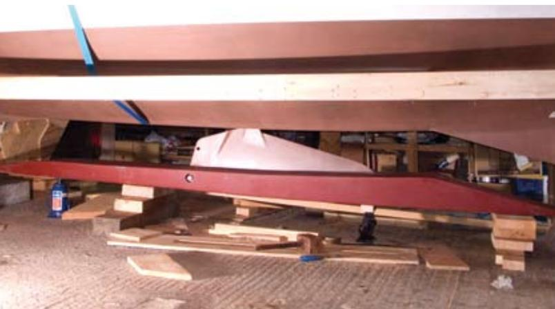
*The cast iron ballast keel, which was positioned under the hull using the ancient Egyptian methods of levers and rollers, is unusual in that it incorporates a slot for the large cast iron centreplate.*
